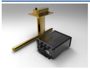
Accurate measurement of temperature, humidity, three-dimensional winds and turbulence on-board the aircraft at spray release height.
